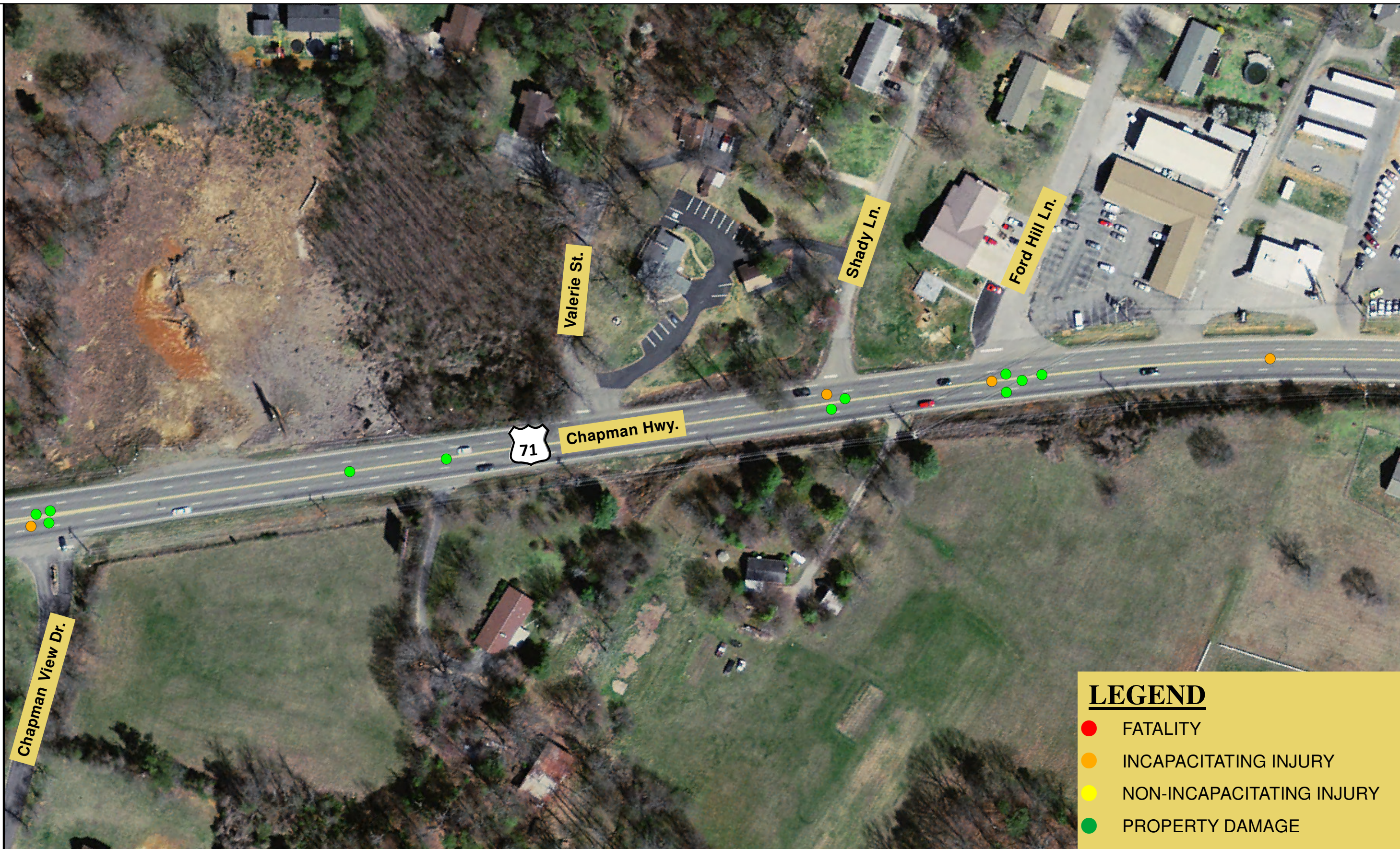
CRASH DIAGRAM S.R. 71 (CHAPMAN HIGHWAY) FROM MACON LANE (L.M. 29.962) TO S.R. 338 / U.S. 411 / S.R. 35 (L.M. 28.790)
